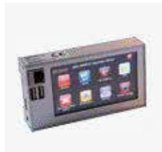
piAx-AM3517 (fanless Single Board Computer with TFT display)
