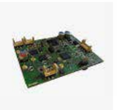
piSmart-Gateway (flexible gateway - applicable as data interface and logger)
