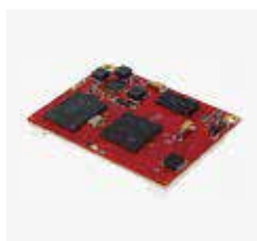
piA-AM335x-PM Low Cost (Cortex™-A8 processor module)
