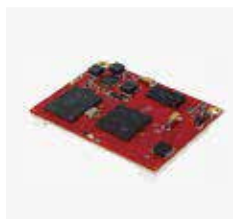
piA-AM335x-PM Industrial (incl. 128Mbit SPI-NOR Flash, 8GB eMMC)
